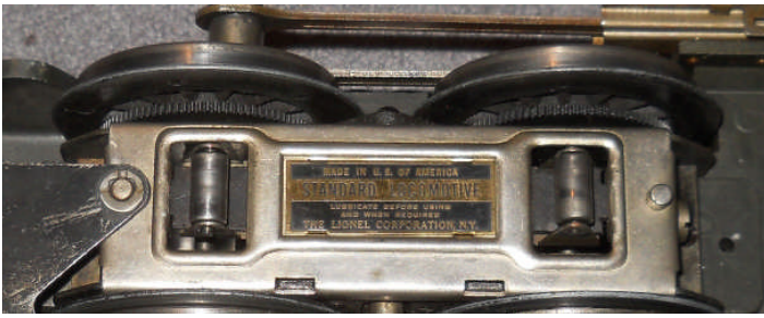
Type 2 Motor from gunmetal No. 392E Locomotive with full nickel trim, Type 5 nickel pickup assembly that is not marked No. 6 as are earlier assemblies. The pickup assembly name plate is marked STANDARD LOCOMOTIVE not BILD-A-LOCO. The studs have slots for the floppy washers.
