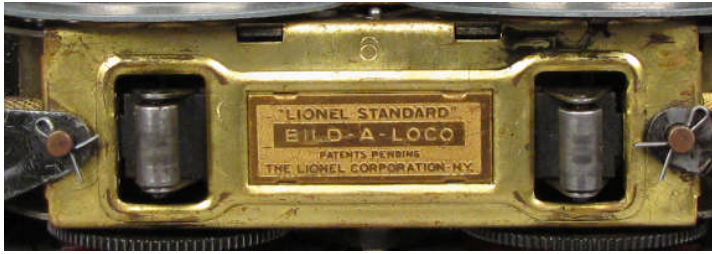
Type 1, "Bild-A-LoCo", gold plate, gold lettering, studs with holes for cotter pins, gold finished bottom assembly. The plate was introduced in 1928 with the Bild-A-LoCo motors, one year before the 390. Source: 390E black, orange stripe, Clement Collection, Ref. 2340
