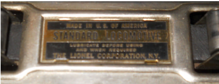
Type 5 nickel finished pickup assembly with pickup plate label "STANDARD LOCOMOTIVE"
