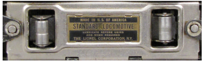
Type 5: "Standard Locomotive" rather than "Bild-A-LoCo", three lines of type below gold band. Trucks fastened by wavy washer rather than cotter pin, nickel finished bottom assembly.. Why did Lionel change the wording? To solve an electrical connection problem, Lionel soldered the pickup assembly connection. This change meant that the motor was no longer a Bild-A-LoCo motor. Source: 385 gunmetal, nickel domes, black drivers. Clement Collection, Ref. IMG 2316. Also found: 392 light gunmetal, Gordon Collection, Ref. 009
