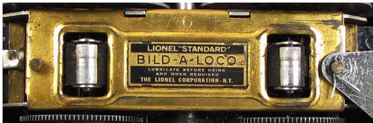
Type 3, "Bild-A-LoCo", three lines of type below gold band, studs with holes for cotter pins, gold finished bottom assembly.. Source: 392 black body, copper domes, Riley Collection, Ref. 392-1
